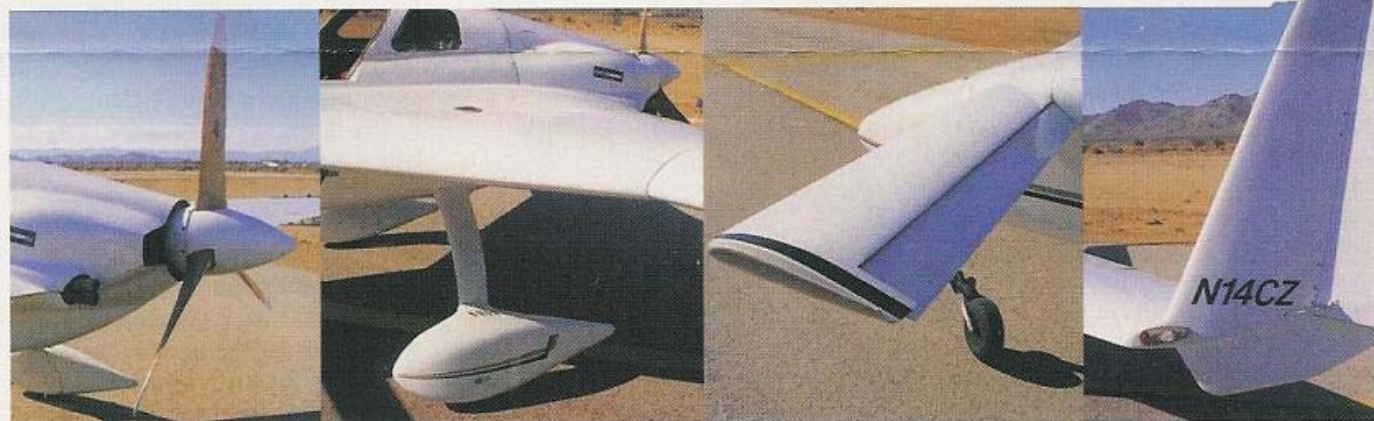
LEFT TO RIGHT: The recommended engine for the Cozy Mark IV is the reliable Lycoming 180-hp engine with a fixed-pitch prop. Like the Long-EZ, the Cozy retracts the nose gear only. The main gear is highly faired to lower the drag considerably. The original canard was much longer (by 6 inches) than the current version. All negative flying habits have been designed out. Nat Puffer redesigned the vertical fins so they protruded beneath the wing as well and solved many early problems.
